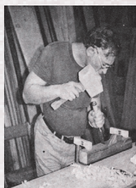
Chiseling out the opening in the sole of a jointer plane.
