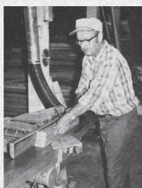
Using the Makita planer/jointer to surface the Cocobolo shoe of a long jointer plane.
